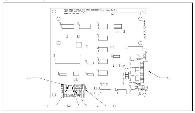
Figure 2.2 Power Board Layout
