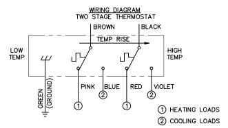
THERMOSTAT OPERATION: DOUBLE POLE, DOUBLE THROW CONTACTS OPERATE SEQUENTIALLY WITH 3'F (1.7'C) NOMINAL SEPARATION ON TEMPERATURE RISE OR FALL. AT TEMPERATURE ABOVE THE SET POINT, LEADS BLACK/VIOLET AND BROWN/BLUE ARE CLOSED. ON TEMPERATURE FALL TO 3'F (1.7'C) (NOMINAL) ABOVE THE SET POINT, LEADS BLACK/RED CLOSE AND BLACK/VIOLET OPEN. ON FURTHER TEMPERATURE FALL TO THE SET POINT, LEADS BROWN/PINK CLOSE AND BROWN/BLUE OPEN.
