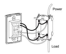
If you wish to connect an external floor temperature sensor, insert the floor sensor cable through one of the two openings on the base and connect the sensor wires to terminals 3 and 4 (no polarity).
