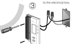
Make sure to firmly tighten the wire connectors for a secure connection. A loose connection can be a fire hazard. Special CO/ALR solderless connectors must be used when connecting with aluminum conductors.
