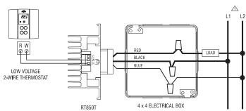
1 You must provide an overload protection and disconnect as required.
