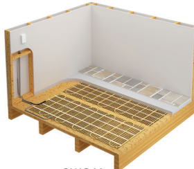
OWC-M: Installation under a 1.5" to 4" concrete topping
