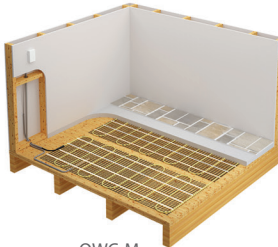
OWC-M: Installation under a 1.5" to 4" concrete topping
