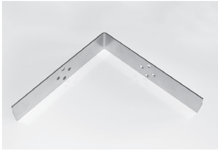
ELB-20: Stainless steel downspout mounting plate to guide and keep heating cable in place at the entrance of a downspout. The heating cable is secured to the plate using plastic fasteners.
