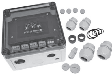
ELTC-14-RTD 1 : Digital display wall temperature control with weather proof plastic enclosure. Power relay of 20A at 90-260V. Including 3-wire RTD (Pt-100) sensing element is 5x50 mm with 16.4 ft (5m) of fluoropolymer lead wires, temperature range 0 °C to 250 °C (32 °F to 482 °F).
