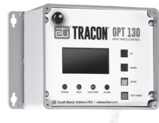
GPT-130: NEMA 4X IP66 electronic single point line sensing heat trace controller 100-277V, 30A c/w built-in 30 mA GFEP and 20 ft. (6 m) lead, 100k ohms at 25 °C (77 °F) thermistor. Range -40 °C to 110 °C (-40 °F to 230 °F).
