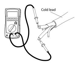
Megger type isolation resistance test
