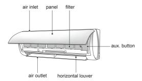
If remote controller is lost or damaged, please use aux. button to turn on or turn off the air conditioner. The operation in details is as below: As shown in the figure, open panel and press aux. button to turn off the air conditioner. When the air conditioner is turned on, it will operate under auto mode.
