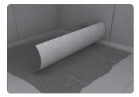
5 Apply a thinset layer to the substrate using a 1/4" x 1/4" square notch trowel. Position the membrane, fleece side down into the thinset. Embed the membrane into the thinset using a float/ roller removing any air pockets.
