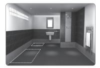
**7** Demarcate the floor to mark the boundaries of fixed elements that cannot be heated.
