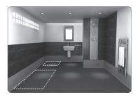
6 Demarcate the floor to mark the boundaries of fixed elements that cannot be heated.
