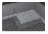
2 Lay the tiles and make sure you have good contact between the adhesive and the membrane. Back-butter the tiles if necessary. When laying the ceramic, ensure the ceramic joints do not lie opposite one of the membrane joints. The two joints must always be offset.
