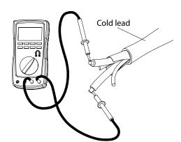
Megger type isolation resistance test
