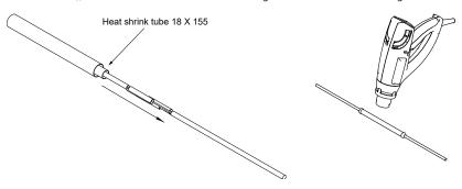
3.3 Repeat the same steps 2.3 to 3.2 for connecting the other extremity of the jumper splice.
