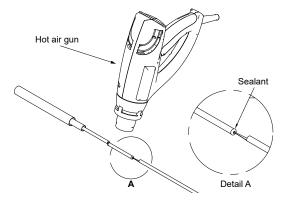
2.6 Insert the 6 x 40 mm heat shrink tube into one of the 65 mm (2 9/16") cut wires.
