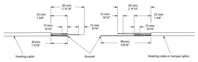
2.3 Insert the 6 x 40 mm into the earlier ground section cut at 90 mm (3 9/16").
