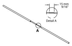
2.8 Insert the 6 x 40 mm heat shrink tube over the connection and make sure it is centered to the mechanical connection. Then heat the entire length of the tube with a hot air gun (do not overheat it), make sure the tube has shrunk enough to see the sealant coming out of both sides.
