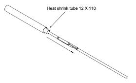
3.1 Heat the entire length of the heat shrink tube with a hot air gun (do not overheat it), make sure the tube has shrunk enough to see the sealant coming out of both sides.
