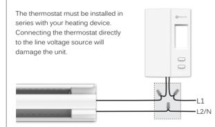
Note: The wires of this thermostat are non-polarized.
