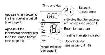
\* To display the set temperature (setpoint), press the **Up** or **Down** button once. The thermostat will display the setpoint instead of the clock for 5 seconds.
